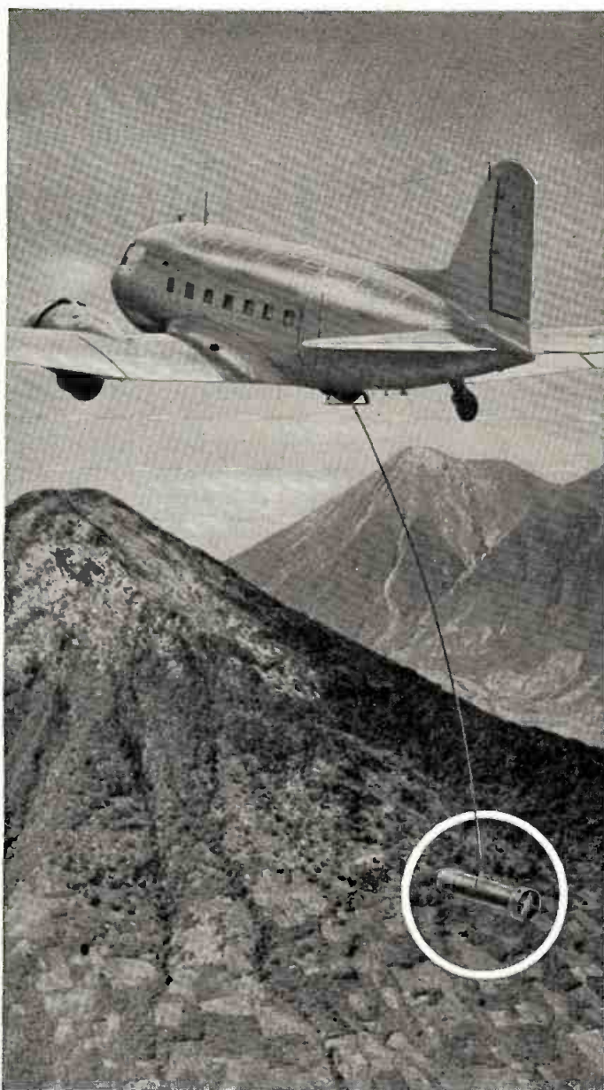
TRAILING BELOW THE OIL EXPLORER'S PLANE , the airborne magnetometer records the earth's magnetic field. Other new ideas and devices are developed by thousands of oil companies in the race to meet oil needs. The driving force—competition; the result—a stronger America—more and better oil products for you.
